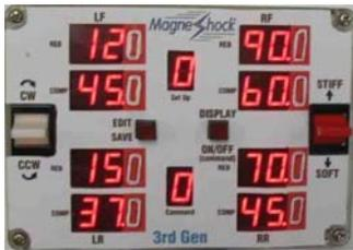
The damping can be adjusted at FIVE (5) velocities: 0, 1/2, 1, 3 & 7 inches/second.
