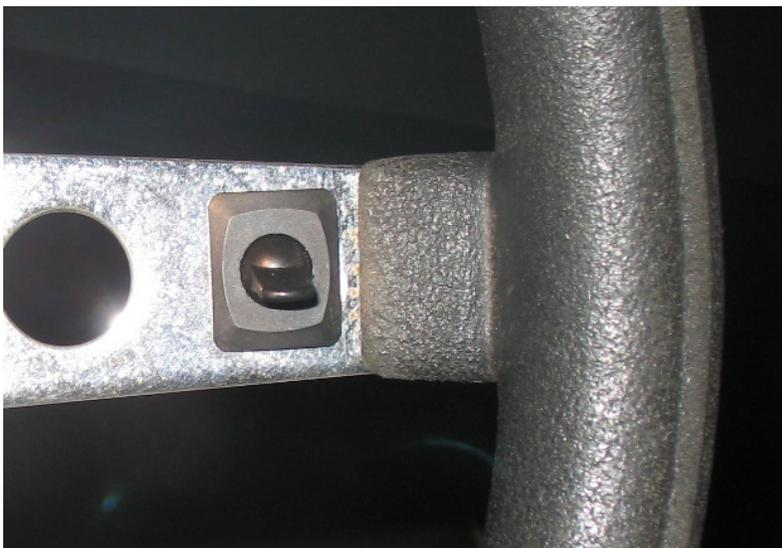
There is also a **2-position bat-handled switch** that can be installed on the steering wheel.
